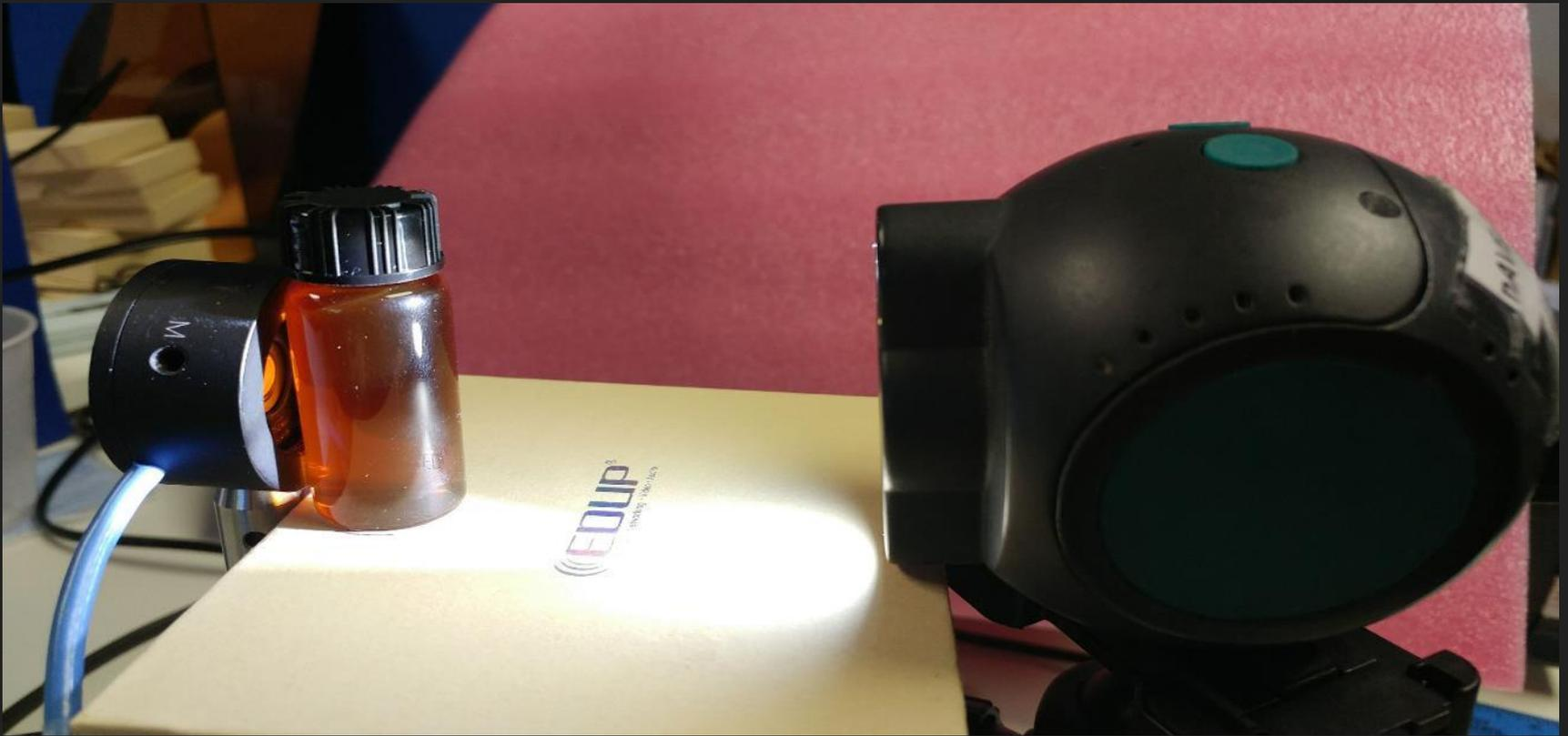
The optical power meter that is used to test the opacity of the coffee concentrations.
